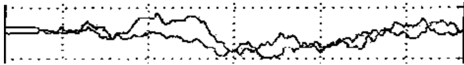
Figure C2: An inconclusive response due to the 3:1 signal to noise rule for a CR not being met and the <25nV noise between waveforms not being met for a RA and a possible response being present. Scales: 150nV / div. 4ms / div
