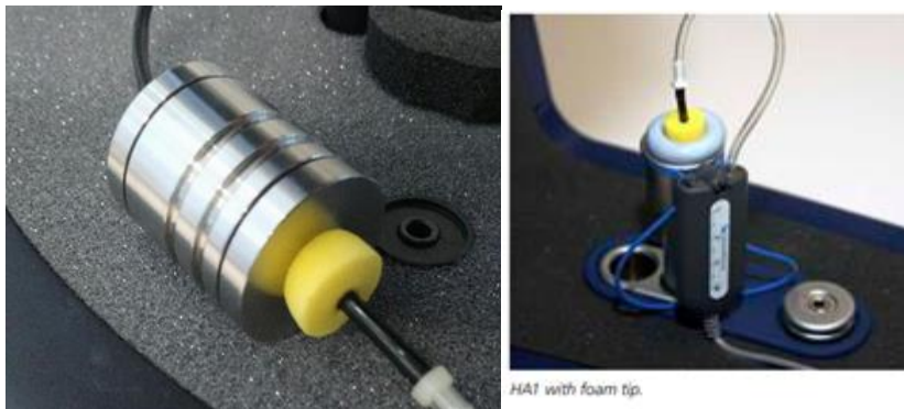
Figure 2: Step by step guide of how to measure an RECD with a closed fitting
