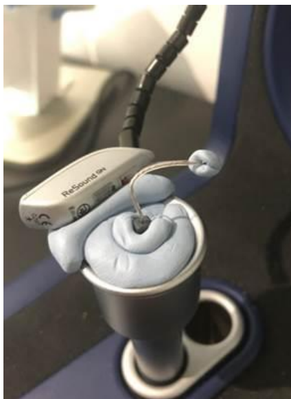
Figure 3: Using putty to replicate the dampening effect of the tubing sitting against a hearing aid wearers head.
