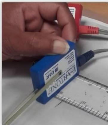
Figure 1. Placement of magnetic field probe over body of Eartone 3a insert.
